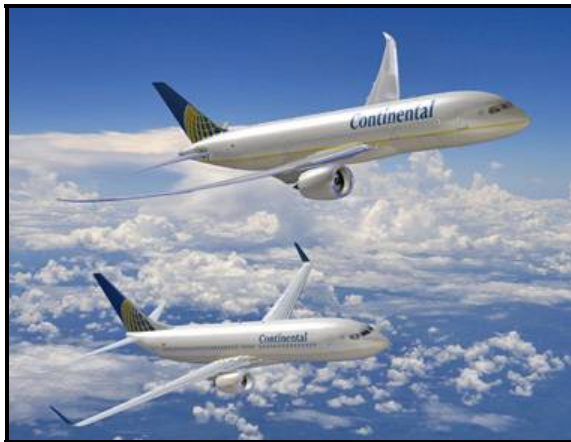
Drag-reducing winglets ( www.Boeingmedia.com )
